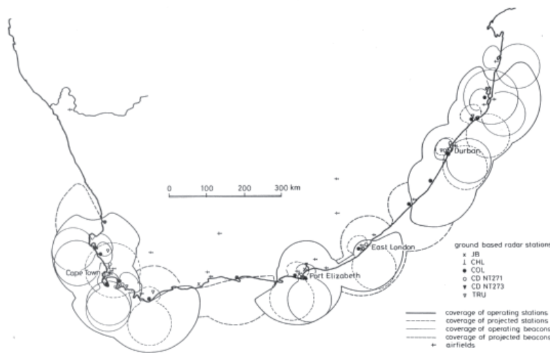
Figure 12. A map showing the position and the predicted coverage from the radar stations around the South African coast.
